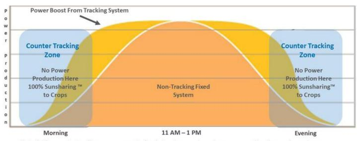
Note 1: The counter tracking zones are not a fixed size, they can be as large or as small as the producer chooses. Note 2: From 11:00am to 1:00pm there is both power production and Sunsharing <sup>™</sup> due to the space between panels
