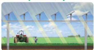
Solar panels are perpendicular to the sunlight and provide partial shading Image Credit: SolAgra
