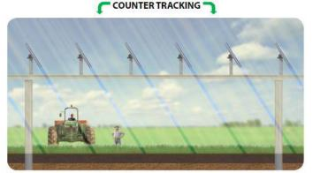
The opposite of Normal Tracking where panels are parallel to the sunlight allowing maximum sunlight on crops
